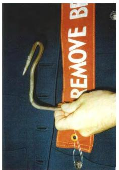
The pin in the picture at the left IS THE REAL ONE! The pin is suppose to be straight. Contact with a rotating propeller on a running Wright R-3350 engine created the multi angles shown. Somehow I managed to keep it with me all these years and it even survived a rather messy divorce in which I lost MUCH military memorabilia (including a couple of photo albums).
