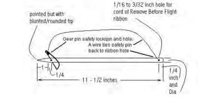
Drawing at right it what an undamaged nose gear pin looks like.
