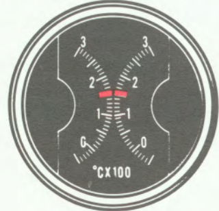
CABIN SUPERCHARGER DRIVE SHAFT REAR BEARING OIL TEMP.
