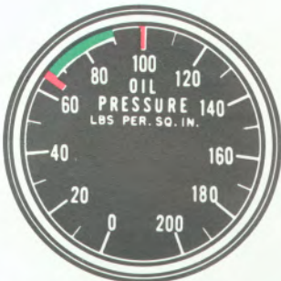
ENGINE OIL PRESSURE (REAR PUMPS)
