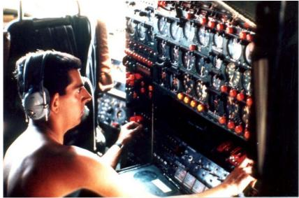
actually have three positions, push to feather, neutral, and pull to unfeather. After a propeller is fully feathered the flight engineer pulls the feather switch back to the neutral position. With the feather switch in neutral the feather pump motor is deactivated.
