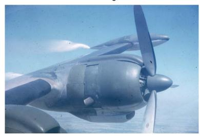
power, to prevent the airplane from maintaining altitude, if the landing gear and flaps are down. Image at left shows the propeller on the number 1 engine feathered. When an engine was lost it was most times necessary to reduce the weight of the airplane by dumping fuel. In this photo you can see fuel being dumped from immediately behind engine #1 and also from the left tip tank.
